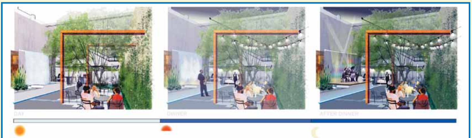
Images depict day-to-evening uses for the vacant lots adjacent to the Downtown Mobile Alliance and the Saenger Theatre along Dauphin Street. The proposed courtyard includes a water well, stormwater planters and rain gardens, retractable movie screen and a seating area.
